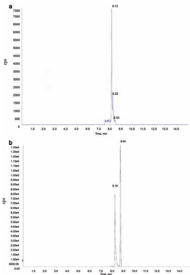
**Figure 6.** (a) MRM ( $m/z$  161.0 $\rightarrow$ 125.0) chromatogram of 2,4-dichlorophenol obtained from 0.5  $\mu\text{g}/\text{mL}$  of the standard mixture in methanol/water (7.66–8.62 min scan window). (b) MRM ( $m/z$  161.0 $\rightarrow$ 125.0) chromatogram of 2,4-dichlorophenol obtained from 1.0  $\mu\text{g}/\text{mL}$  of the standard mixture in methanol/water (7.66–8.66 min scan window).
