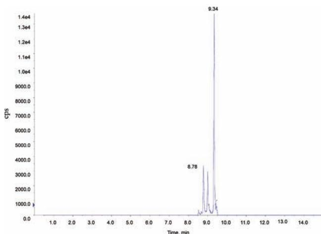
Figure 4. MRM ( $m/z$  197.0 $\rightarrow$ 161.0) chromatogram of 2,4,5-trichlorophenol obtained from 1.0  $\mu\text{g}/\text{mL}$  of the standard mixture in methanol/water.
