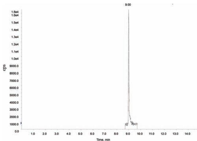
Figure 5. MRM ( $m/z$  197.0 $\rightarrow$ 161.0) chromatogram of 2,4,5-trichlorophenol obtained from 1.0  $\mu\text{g}/\text{mL}$  of the standard in methanol/water.
